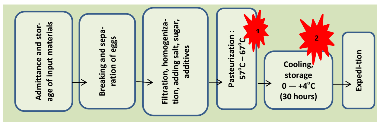
Figure 4 – The major stages of the technological chain and the envisaged CCP for this industry
